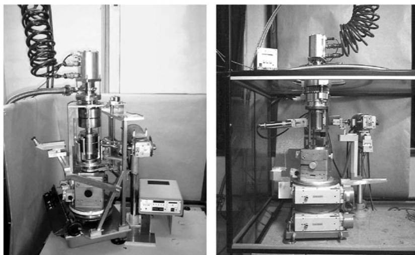
Figure 1. View of the vertical Weissenberg camera (left) and the Huber diffractometer (right), each with their cryostat.
